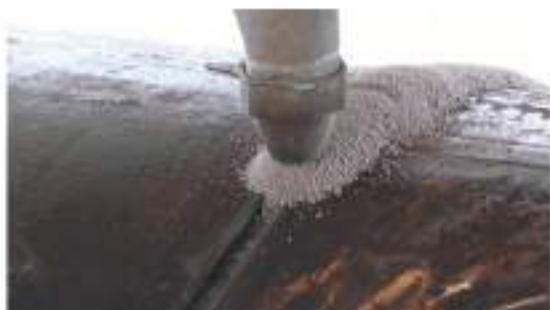
**Submerged-arc welding (SAW)** involves the formation of an arc between a continuously fed electrode and the workpiece. A blanket of powdered flux, which generates a protective gas shield and a slag (and may also be used to add alloying elements to the weld pool), protects the weld zone. A shielding gas is not required.
