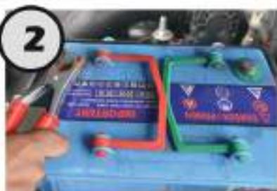
REMOVE THE CLAMPS OF (+) POSITIVE AND (-) NEGATIVE TERMINALS OF THE BATTERY.
