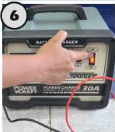
SWITCH TO CORRECT VOLTAGE SETTING
